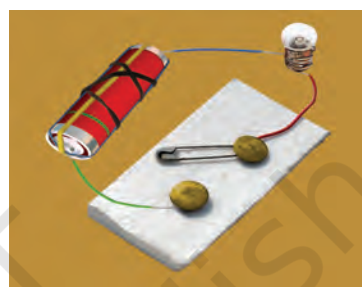
Fig 12.9 An electric circuit with a switch
